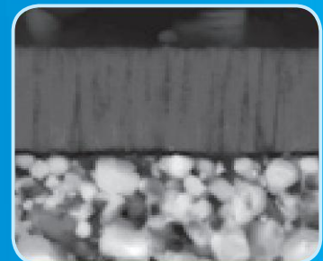
PVD coating organization structure of cermet
